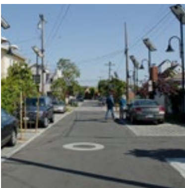
Narrow two-way streets with on-street parking require drivers to take turns driving in each direction, forcing slower traffic speeds.
